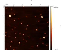
AFM ex-situ analysis (scan area 5x5 μm<sup>2</sup>)
