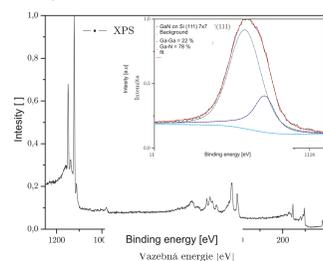
XPS spectra of a GaN film (the inset shows the Ga 2p peak fit with the parameters listed in the table below)
