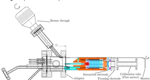
Model of the ion-atom beam source and the cross section of the source body.
