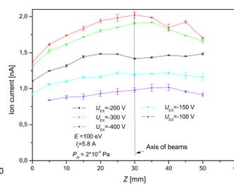
Ion beam profiles for various extraction potential.
