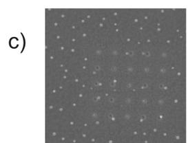
The selective growth of GaN droplets on the Si(111) 7x7 substrate pre-patterned by FIB (see Fig. b)
