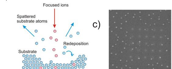
Principle of milling by FIB
