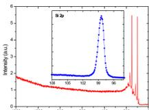
XPS spectra of Si(111) 7x7 structure after flash annealing
