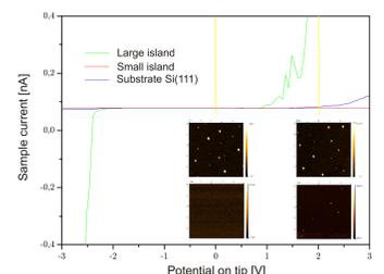
Local conductivity of GaN droplets measured by C-AFM
