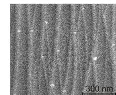
The detail of GaN droplets growing at room temperature on Si(111) 7x7 substrate measured by SEM (FEI company)
