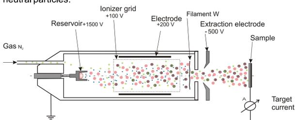
Schematic of the ion-atom beam source generating hyperthermal ions (30 - 200 eV).
