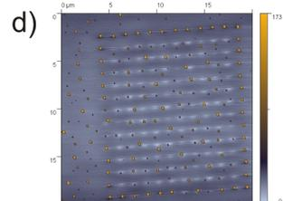
Array of GaN grown on Si(111) 7x7 substrate pre-patterned by FIB
