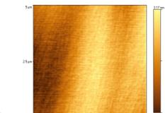
AFM ex-situ analysis of Si(111) 7x7 structure after flash annealing
