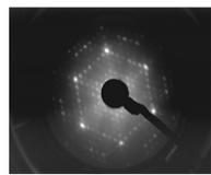
LEED pattern of Si(111) 7x7 structure after flash annealing
